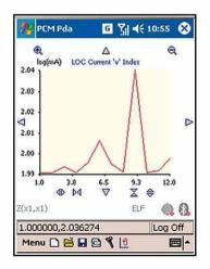
The Radiodetection Survey software incorporates GPS information and shows the mapped data in a variety of formats as well as allowing comparisons between new and old mapping surveys.
